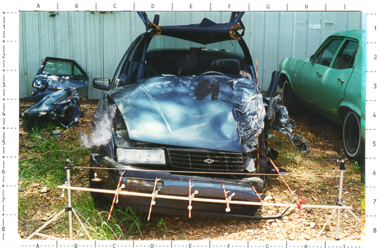
# 30 -- Frontal view of 1991 Chevrolet Corsica's front left damage with contour gauge present
